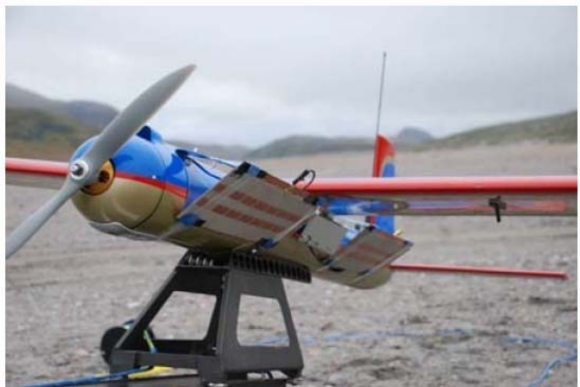
Figure 17. The MicroSAR mounted onto the electric Silver Fox UAV prior to launch in Greenland.
